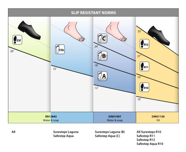
A sustainable, lifetime performance as a result of particles throughout the matrix of the product is the requirement to comply with EN 13845. This standard specifies the requirements that must be met to ensure durable slip resistance in varying degrees of usage intensity. All Step floors comply with EN13845.
